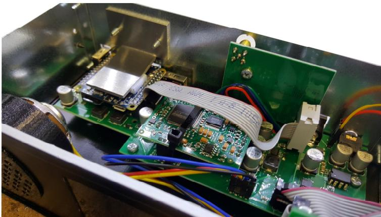
Place ribbon cable on option connector as shown on next photo.
